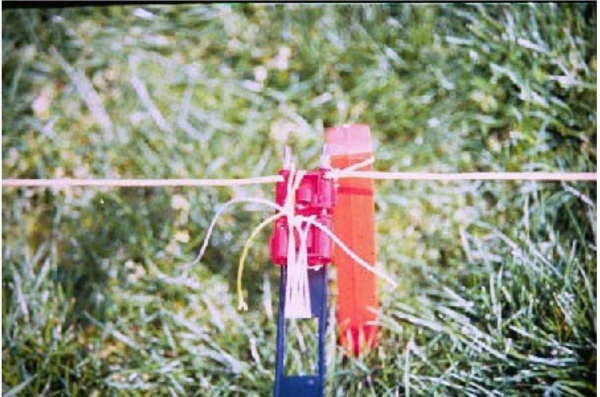
10infeed shows the manner of connecting the antenna system to 3/4 inch ladder-line by the use of dual-banana plugs.
