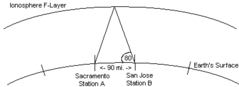
\ distance = 90 miles / Vertical radiation angle to reach from station "A" to "B" = 80 Degrees
